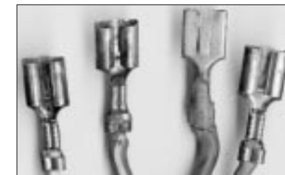
Connector removed from shell or gangplug. Carefully squeeze the rounded sides so they make better contact with the spade - not shown.
