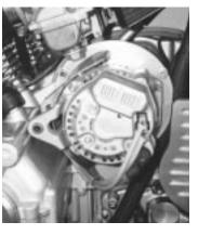
conditions with no oil leaks or funny noises. The engine was occasionally test over-revved with no ill effects. The voltmeter stayed on charge from 1500 rpm and up.
